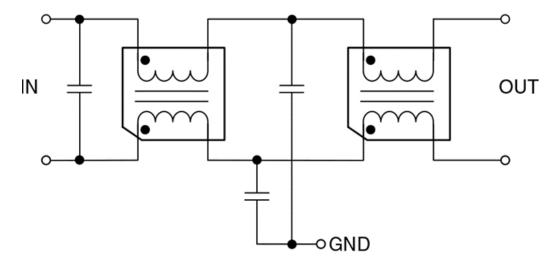
Figure 5. Internal Schematic
