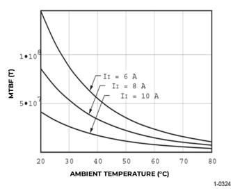
Figure 4. MTBF vs Ambient temperature for 6A, 8A, and 10A Input Current
