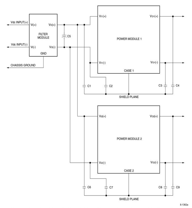
Note: C1 through C4 and C6 through C9 can be 0.01  $\mu$ F to 0.1  $\mu$ F. Select the voltage rating to meet input-to-output isolation requirements. C5 should be the recommended value indicated in the power module data sheet.
