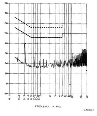
Figure 10. JW075A5 Conducted Noise with Filter
