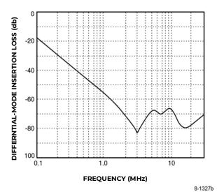
Figure 3. Typical Differential-Mode Insertion Loss in a 50  $\Omega$  Circuit
