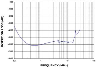
Figure 3: Typical Differential-Mode Insertion Loss in a  $50\Omega$  circuit. (Standard Version, 100MHz Axis max.)
