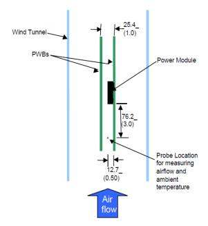
Figure 12. Thermal Test Set-up.
