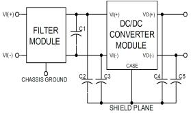
Figure 9. Schematic diagram showing recommended connection of the FLT012A0 filter module with metal cased DC/DC converter modules.
