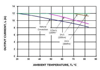
Figure 5. Derating Output Current versus Local Ambient Temperature and Airflow.
