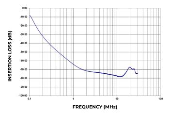
Figure 1: Typical Common-Mode Insertion Loss in a  $50\Omega$  circuit (Standard Version, 100MHz Axis max.)
