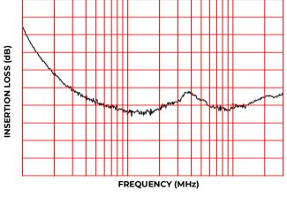
Figure 4.: Typical Differential-Mode Insertion Loss in a 50  $\Omega$  circuit. (-11 Option, 30MHz Axis max.)
