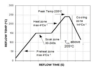
Figure 15 Reflow Profile for Tin/Lead (Sn/Pb) process.
