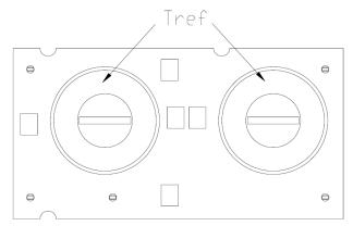
Figure 13. T<sub>ref</sub> Temperature measurement location.
