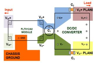
Figure 8. Diagram showing recommended layout of the FLT012A0 filter module with open-frame DC/DC converter modules.
