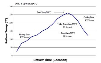
Figure 17. Recommended linear reflow profile using Sn/Aq/Cu solder.
