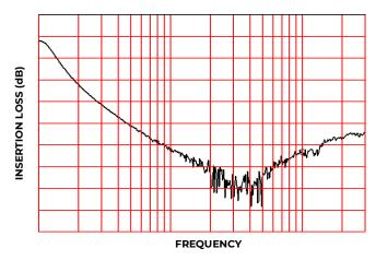
Figure 2: Typical Common-Mode Insertion Loss in a 50  $\Omega$  circuit. (-11 Option, 30MHz Axis max.)
