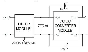
Figure 7. Schematic diagram showing recommended connection of the FLT012A0 filter module with open frame DC/DC converter modules.
