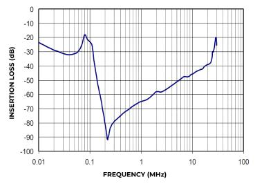
Figure 2. Typical Differential-Mode Insertion Loss in a 50  $\boldsymbol{\Omega}$  circuit.
