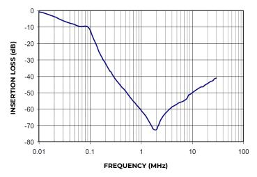
Figure 1: Typical Common-Mode Insertion Loss in a  $50\Omega$  circuit
