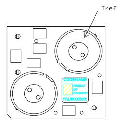
Figure 11. T<sub>ref</sub> Temperature measurement location.
