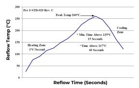
Figure 15. Recommended linear reflow profile using Sn/Ag/Cu solder.
