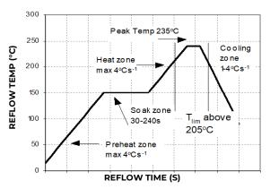
Figure 13 Reflow Profile for Tin/Lead (Sn/Pb) process.
