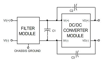
Figure 5. Schematic diagram showing recommended connection of the FLT007A0Z filter module with open frame DC/DC converter modules.
