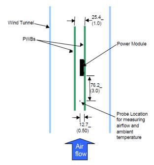
Figure 10. Thermal Test Set-up.
