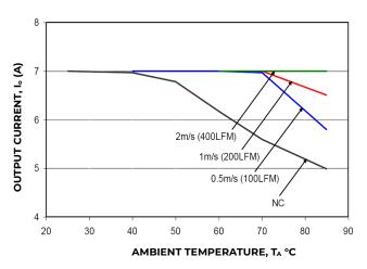
Figure 3. Derating Output Current versus Local Ambient Temperature and Airflow.
