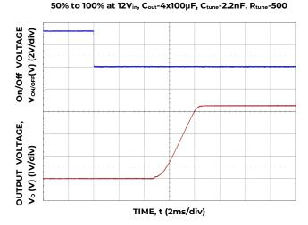
Figure 29. Typical Start-up Using On/Off Voltage  $(I_0 = I_0, m_{ax})$ .
