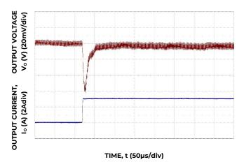
Figure 28. Transient Response to Dynamic Load Change from
