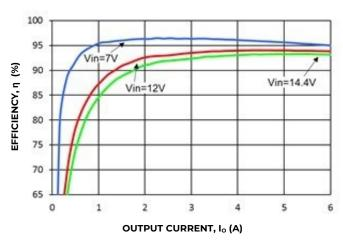
Figure 31. Converter Efficiency versus Output Current.
