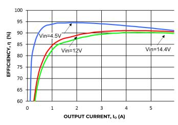
Figure 19. Converter Efficiency versus Output Current.
