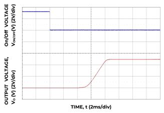
Figure 35. Typical Start-up Using On/Off Voltage  $(I_0 = I_{07 \text{ max}}).$
