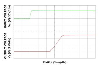
Figure 36. Typical Start-up Using Input Voltage ( $V_{IN} = 12 V$ ,  $I_0 = I_0$ , max.)
