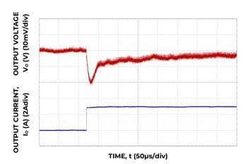
Figure 4. Transient Response to Dynamic Load Change from 5% to 100% at 12 Vin,  $C_{out}$ - 2x 330µF, 6x 100µF,  $C_{tune}$  - 10µF,  $R_{tune}$ - 500
