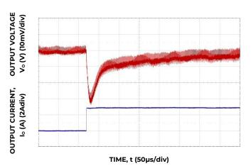
Figure 10. Transient Response to Dynamic Load Change from 50% to 100% at 12Vin, Cout-1x330 $\mu$ F, 4x100 $\mu$ F, Ctune-4.7nF, Rtune-500
