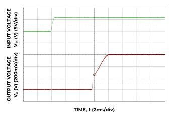
Figure 6. Typical Start-up Using Input Voltage ( $V_{IN} = 12 V I_0 = I_{O, max.}$ )
