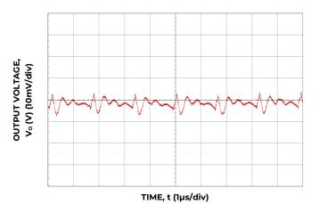
Figure 3. Typical Output Ripple and Noise, ( $C_o = 88 \mu$ F Ceramic,  $V_{IN} = 12 V I_o = I_{o, max.}$ )
