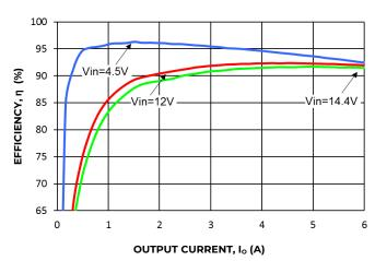
Figure 25. Converter Efficiency versus Output Current.
