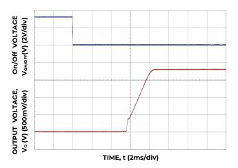
Figure 17. Typical Start-up Usin On/Off Voltage (Io = Io, max).
