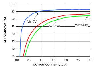
Figure 31. Converter Efficiency versus Output Current.
