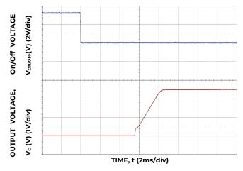
Figure 23. Typical Start-up Using On/Off Voltage (I<sub>o</sub> = I<sub>o</sub>, <sub>max</sub>).
