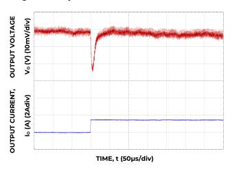
Figure 16. Transient Response to Dynamic Load Change from 5% to 100% at 12 Vin, Cout- 4x 100µF, Ctune - 4.7nF, Rtune- 400
