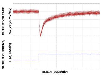
Figure 28. Transient Response to Dynamic Load Change from 5% to 100% at 12 Vin, Cout- 2x 100μF, Ctune - 1nF, Rtune- 500
