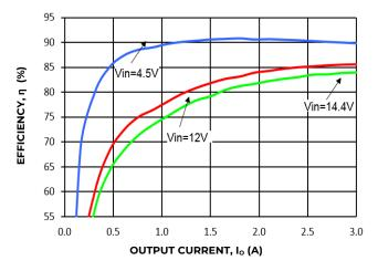
Figure 7. Converter Efficiency versus Output Current.
