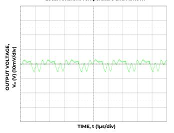
Figure 15. Typical Output Ripple and Noise, ( $C_o = 88 \mu F$  Ceramic,  $V_{IN} = 12 V$   $I_0 = I_0$ ,  $_{max.}$ )
