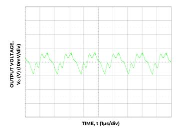
Figure 33. Typical Output Ripple and Noise, ( $C_o$  = 88  $\mu$ F Ceramic,  $V_{IN}$  = 12  $V_{Io}$  =  $I_{O, max.}$ )
