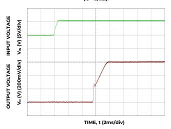
Figure 6. Typical Start-up Using Input Voltage ( $V_{IN} = 12 V I_0 = I_{O, max.}$ )
