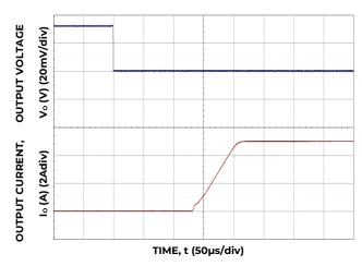
Figure 34. Transient Response to Dynamic Load Change from 5% to 100% at 12 Vin, Cout- 1x 100µF, Ctune - 680pF, Rtune- 500
