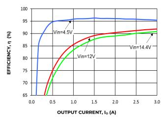
Figure 25. Converter Efficiency versus Output Current.
