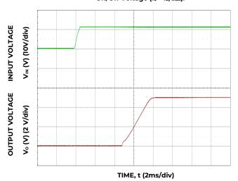
Figure 36. Typical Start-up Using Input Voltage ( $V_{IN} = 12 \text{ V}, I_0 = I_0, max.$ )
