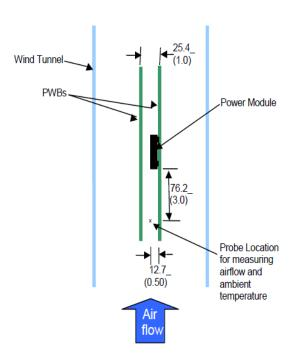
Figure 46. Thermal Test Setup.
