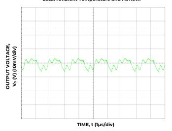
Figure 21. Typical Output Ripple and Noise, ( $C_o = 88 \mu F$  Ceramic,  $V_{IN} = 12 V l_o = l_o, max.$ )
