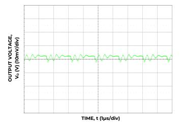
Figure 3. Typical Output Ripple and Noise, ( $C_0 = 88 \mu F$  Ceramic,  $V_{IN} = 12 V I_0 = I_0$ , max.)
