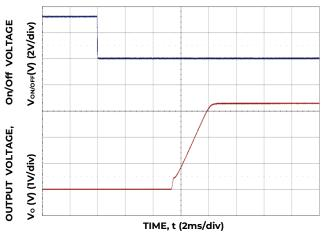
Figure 29. Typical Start-up Using On/Off Voltage (I<sub>o</sub> = I<sub>o</sub>, max).
