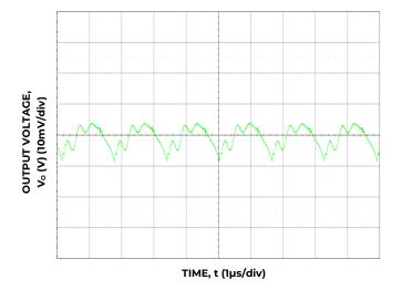
Figure 27. Typical Output Ripple and Noise, ( $C_0 = 88 \mu F$  Ceramic,  $V_{IN} = 12 V I_0 = I_0, max.$ )
