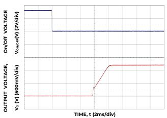
Figure 11. Typical Start-up Using On/Off Voltage (I<sub>o</sub> = I<sub>o</sub>, max).
