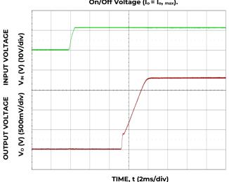
Figure 18. Typical Start-up Using Input Voltage ( $V_{IN} = 12 \text{ V}$ ,  $I_0 = I_0$ , max.)
