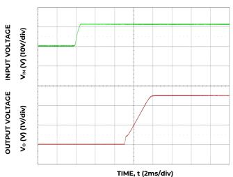
Figure 24. Typical Start-up Using Input Voltage ( $V_{IN} = 12 \text{ V}$ ,  $I_0 = I_0$ , max.)
