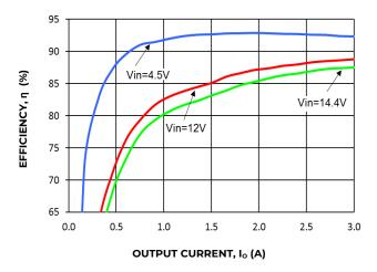
Figure 13. Converter Efficiency versus Output Current.
