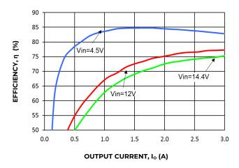
Figure 1. Converter Efficiency versus Output Current.
