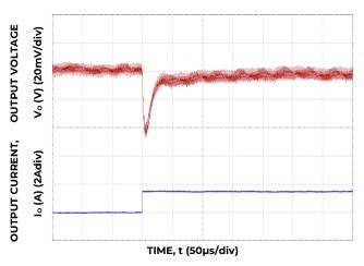
Figure 22. Transient Response to Dynamic Load Change from 5% to 100% at 12 Vin, Cout- 2x 100µF, Ctune - 1.5nF, Rtune- 500
