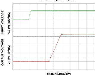
Figure 30. Typical Start-up Using Input Voltage ( $V_{IN} = 12 \text{ V}, I_0 = I_0, max.$ )
