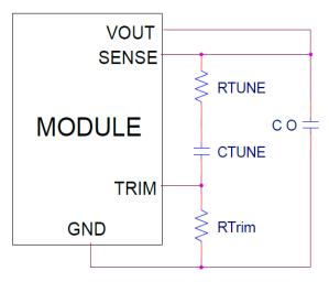
Figure. 45. Circuit diagram showing connection of  $R_{\text{TUNE}}$  and  $C_{\text{TUNE}}$ to tune the control loop of the module.
