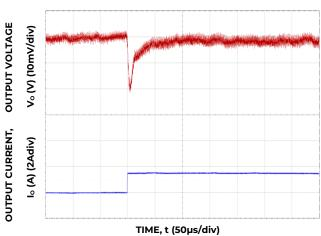
Figure 10. Transient Response to Dynamic Load Change from 5% to 100% at 12 Vin, Cout- 4x 100µF, Ctune - 4.7µF, Rtune- 400
