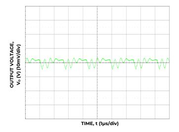
Figure 9. Typical Output Ripple and Noise, ( $C_0 = 88 \mu F$  Ceramic,  $V_{IN} = 12 V I_0 = I_0$ , max.)
