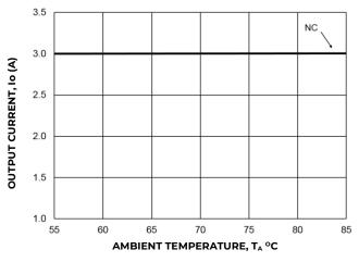
Figure 32. Derating Output Current versus Local Ambient Temperature and Airflow.
