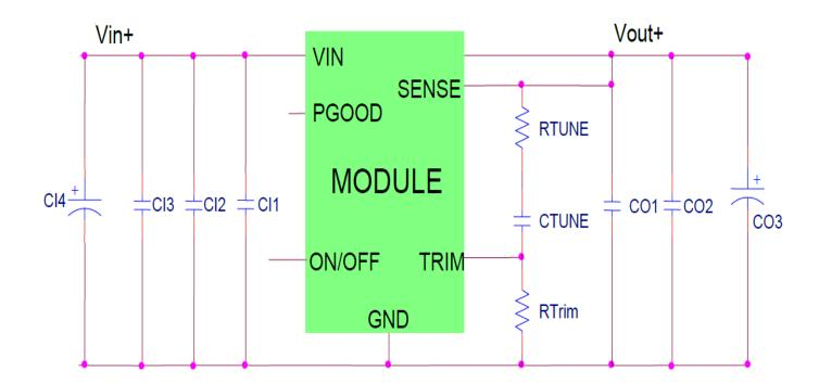
CII Decoupling cap – 0.1µF/16V ceramic capacitor (e.g. Murata GRM155R71C104KA88D)
