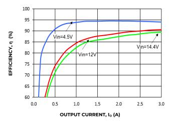
Figure 19. Converter Efficiency versus Output Current.
