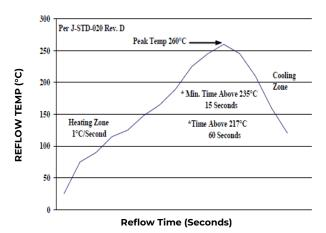
Figure 48. Recommended linear reflow profile using Sn/Ag/Cu solder.
