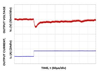
Figure 4. Transient Response to Dynamic Load Change from 5% to 100% at 12 Vin, Cout- 2x 330 $\mu$ F, 6x 100 $\mu$ F, Ctune - 10 $\mu$ F, Rtune- 500 V<sub>IN</sub>=5V.
