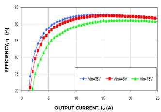
Figure 1. Converter Efficiency versus Output Current.
