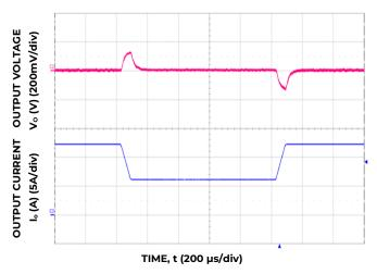
Figure 3. Transient Response to 0.1A/ $\mu S$  Dynamic Load Change from 25% to 50% to 25% of full load,
