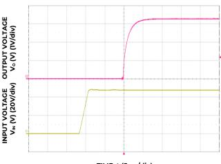
TIME, t (5ms/div) Figure 6. Typical Start-up Using Input Voltage ( VIN = VIN,NOM, Io = Io, max).
