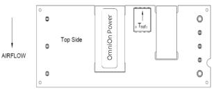
Figure 13a. T<sub>ref</sub> 1 Temperature Measurement Location for Open Frame Module.
