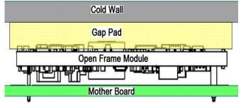
Figure 16. Cold Wall Mounting
