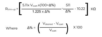
For example, to trim-up the output voltage of the module by 5% to 3.465V,  $R_{trim-up}$  is calculated is as follows:  $\Delta\% = 5$
