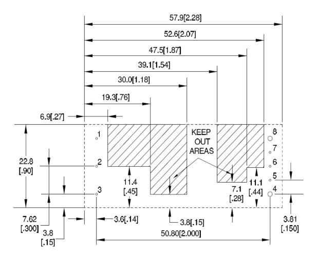
TH Recommended Pad Layout (Component Side View)
