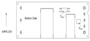
Figure 13b. T<sub>ref 2</sub> and T<sub>ref 3</sub> Temperature Measurement Locations for Open Frame Module.
