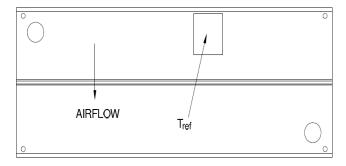
Figure 14. T<sub>ref</sub> Temperature Measurement Location for Module with Heatplate.
