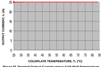
Figure 17. Derated Output Current versus Cold Wall Temperature with local ambient temperature around module at 85C;  $V_{in}$ =48V.
