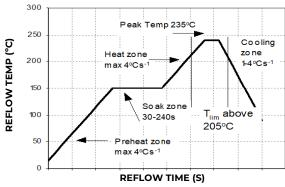
Figure 19. Reflow Profile for Tin/Lead (Sn/Pb) process.
