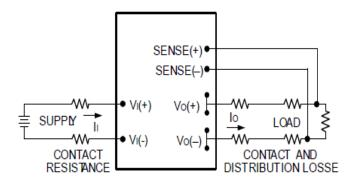
Figure 11. Circuit Configuration for remote sense.
