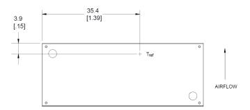
Figure 14. T<sub>ref</sub> Temperature Measurement Location for Module with Heatplate.
