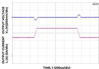
Figure 4. Transient Response to 0.1A/ $\mu$ S Dynamic Load Change from 50% to 75% to 50% of full load,  $V_{in}$ =48V
