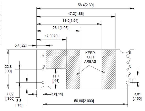
TH Recommended Pad Layout (Component Side View)
