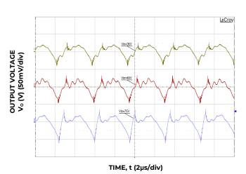
Figure 2.Typical output ripple and noise (I<sub>o</sub> = I<sub>o, max</sub>).
