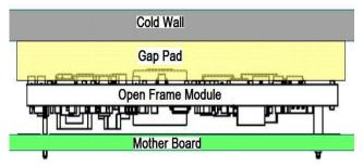
Figure 18. Cold Wall Mounting
