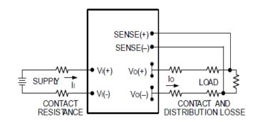
Figure 11. Circuit Configuration for remote sense .
