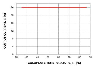
Figure 19. Derated Output Current versus Cold Wall Temperature with local ambient temperature around module at 85C;  $V_{\rm in}$ =48V.
