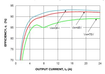
Figure 1. Converter Efficiency versus Output Current.
