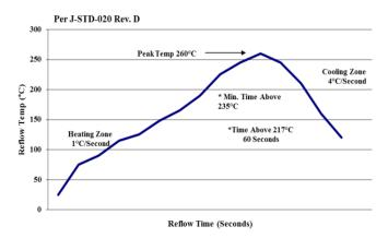
Figure 23. Recommended linear reflow profile using Sn/Ag/Cu solder.
