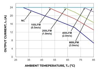
Figure 15. Output Current Derating for the Open Frame Module; Airflow in the Transverse Direction from  $V_{out}$  (-) to  $V_{out}$  (+);  $V_{IN}$  =48V,  $V_0$ = 5.0V.
