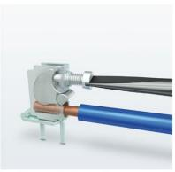
Cable routing and actuation of the terminal block screw on one level – front screw connection for narrow device fronts and PCB racks. The conductor is reliably clamped by the force-increasing swiveling movement of the angled pressure plate.
