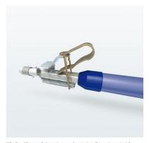
Whether it's a push-in spring or a leg spring, the spring principle makes for quick, tool-free conductor connection. Simply insert the solid conductors and conductors with ferrules into the push-in terminal point and release using a screwdriver. When connecting and releasing finely stranded conductors without ferrules, the terminal point can also be opened using a screwdriver.
