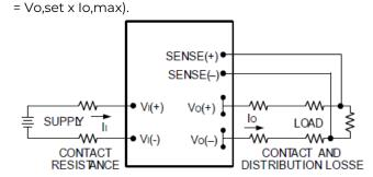
Figure 11. Circuit Configuration for remote sense.
