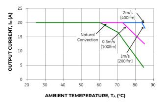
Figure 21. Output Current Derating for the Module with -18 Heatplate; Airflow in the Transverse Direction from  $V_{out}(-)$  to  $V_{out}(+)$ ; $V_{IN}$  =24V
