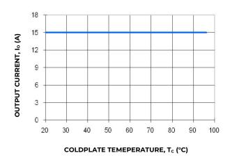
Figure 23. Derated Output Current versus Cold Wall Temperature with local ambient temperature around module at 85°C;  $V_{\text{IN}}$  =24V or 48V.
