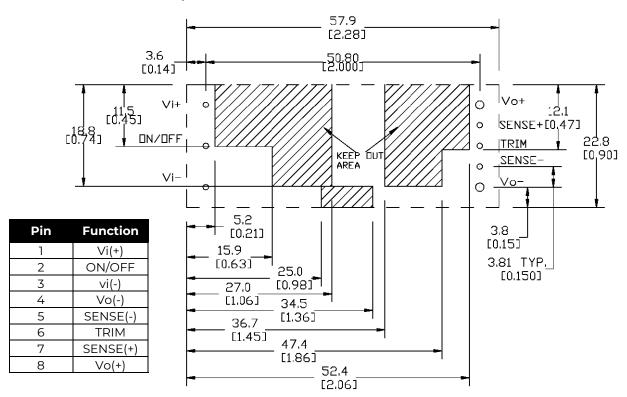
TH Recommended Pad Layout (Component Side View)
