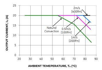
Figure 17. Output Current Derating for the Module with Heatplate; Airflow in the Transverse Direction from V<sub>out</sub>(-) to V<sub>out</sub>(+);V<sub>IN</sub> =48V
