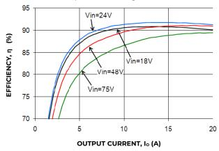
Figure 1. Converter Efficiency versus Output Current.
