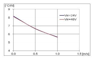
Figure 15. Thermal Resistance for the Open Frame Module; Airflow in the Transverse Direction from Vout(-) to  $V_{out}(+)$ ;  $V_{IN}$  =24V or 48V,  $V_{o}$ =3.3V.
