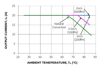
Figure 18. Output Current Derating for the Module with -18 Heatplate; Airflow in the Transverse Direction from  $V_{out}(-)$  to  $V_{out}(+)$ ;  $V_{in}$  =48V.
