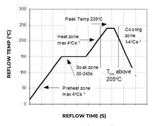
Figure 25. Reflow Profile for Tin/Lead (Sn/Pb) process.
