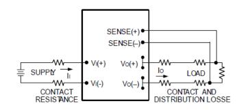
Figure 11. Circuit Configuration for remote sense.
