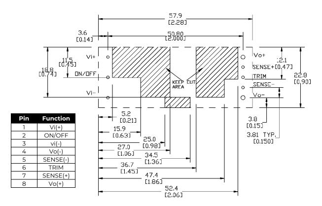
TH Recommended Pad Layout (Component Side View)
