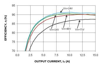
Figure 1. Converter Efficiency versus Output Current.
