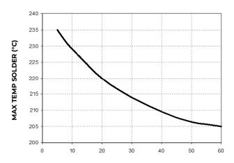
Figure 26. Time Limit Curve Above 20°C for Tin/Lead (Sn/Pb) process
