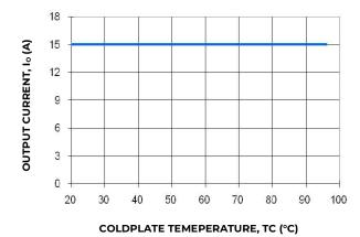
Figure 23. Derated Output Current versus Cold Wall Temperature with local ambient temperature around module at 85C; V<sub>IN</sub> =24V or 48V.
