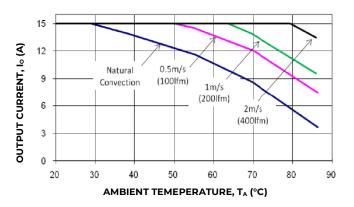
Figure 20. Output Current Derating for the Module with Heatplate; Airflow in the Transverse Direction from  $V_{out}(-)$  to  $V_{out}(+)$ ;  $V_{IN}$  =24V,  $V_0$ =5.0V.
