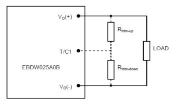
Figure 17. Circuit Configuration to Trim Output Voltage.
