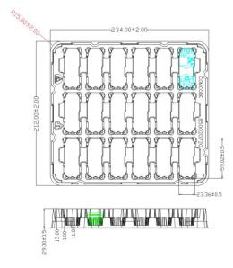
Open Frame Through Hole Pin Module Tray
