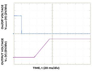
Figure 4. Typical Start-Up Using Remote On/Off with Vin applied, negative logic version shown.
