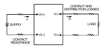
Figure 14. Output Voltage and Efficiency Test Setup.
