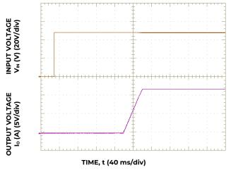
Figure 3. Typical Start-Up Using Vin with Remote On/Off enabled, negative logic version shown. Page 7
