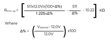
For example, to trim-up the output voltage of the module by 5% to 12.6V, R<sub>trim-up</sub> is calculated is as follows:
