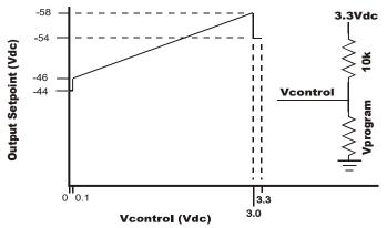
An open circuit on this pin reverts the voltage level back to the original setting..
