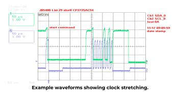
**Communications speed:** Both 100kHz and 400kHz clock rates are supported. The power supplies default to the 100kHz clock rate.
