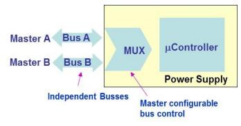
Diagram showing the dual I<sup>2</sup>C bus system.
