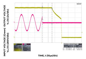
Figure 7. Typical Hold-up Waveforms (V<sub>IN</sub> = 230V, 100% Load)
