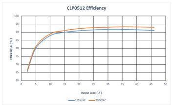
Figure 1: Power Supply Efficiency Versus Output Current
