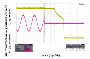
Figure 6. Typical Hold-up Waveforms (V<sub>IN</sub> = 115V<sub>ac</sub>, 100% Load)
