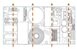
Fig. 2. Preferred airflow direction for cooling
