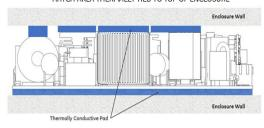
Fig. 1. Example arrangement of the CLP0512 for sealed enclosure applications.
