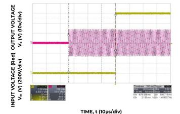
Figure 4. Typical Start-up (V<sub>IN</sub> = 90V<sub>ac</sub>, Full Load)
