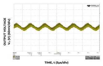
Figure 3. Typical output ripple and noise (V<sub>IN</sub> = 115V<sub>AC</sub>, 100% load )
