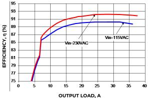
Figure 1. Power Supply Efficiency Versus Out Current
