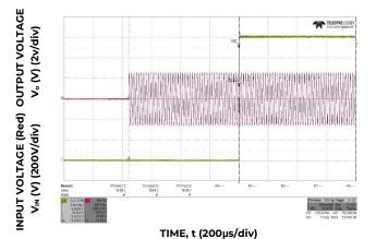
Figure 6. Typical Start-up (V<sub>IN</sub> = 230V<sub>AC</sub>, Full Load)
