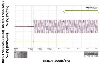
Figure 5. Typical Start-up (V<sub>IN</sub> = 90V<sub>AC</sub>, Full Load)
