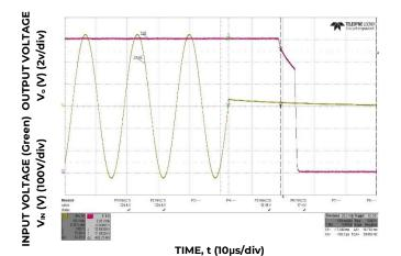
Figure 8. Typical Hold-up (V<sub>IN</sub> = 230V, 100% Load)
