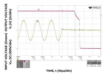
Figure 7. Typical Hold-up  $(V_{IN} = 115V, 100\% Load)$
