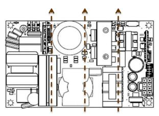
Fig. 9 Preferred airflow direction for cooling.
