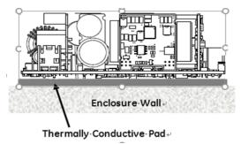
Note that the Ambient Temperature shown in Table 1 is that outside the sealed enclosure, the unit may see higher ambient temperatures.
