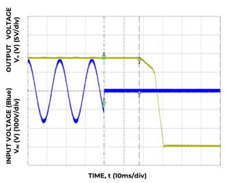
Figure 9. Typical Hold-up waveforms – ..Z02A version  $(V_{IN} = 115V, 100\% \text{ load}).$
