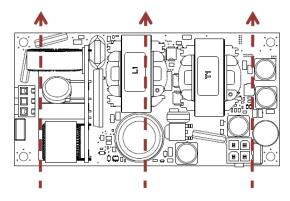
Fig. 12. Preferred airflow direction for cooling.
