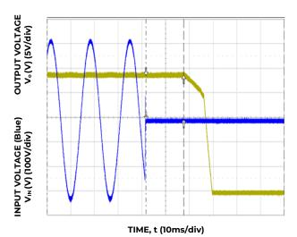
Figure 8. Typical Hold-up waveforms - all except ..Z02A version ( $V_{IN}$  = 115V, 100% load). ( $V_{IN}$  = 230V, 100% load).
