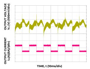
Figure 4. Transient Response to Dynamic Load Change from 50% to 100% at  $V_{\rm IN}$  = 230 $V_{\rm ac}$ .
