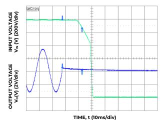
Figure 8. Typical Hold-up waveforms (V<sub>IN</sub> = 230V, 100% load).
