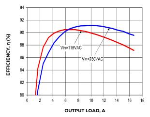
Figure 1. Power Supply Efficiency versus Output Current.
