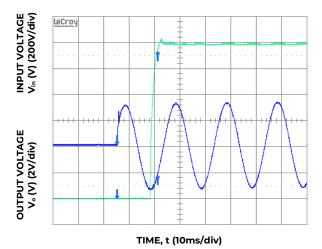
Figure 6. Typical Start-up (V<sub>IN</sub> = 230V<sub>ac</sub>)
