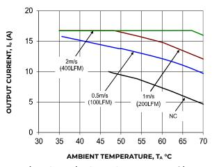
Figure 2. Derating Output Current versus Ambient Temperature and Airflow. Data shown for 115 $V_{\rm AC}$  in, at 230 $V_{\rm AC}$  in derating is the same or better. For derating at other input voltages, consult the OmniOn Technical representative.
