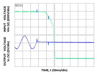
Figure 7. Typical Hold-up waveforms (V<sub>IN</sub> = 115V, 100% load).
