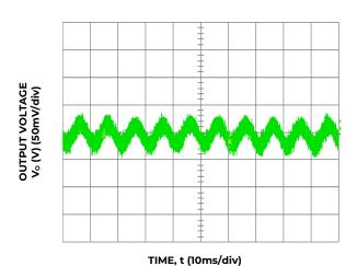
Figure 3. Typical output ripple and noise ( $V_{\text{IN}}$  = 230 $V_{\text{ac}}$ , 100% load ).
