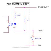
Fig. 9. Schematic showing ON/OFF circuitry.
