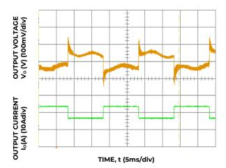
Figure 4. Transient Response to Dynamic Load Change from 50% to 100% at  $V_{\rm IN}$  = 230 $V_{\rm ac}$
