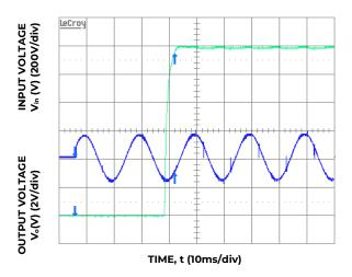
Figure 5. Typical Start-up ( $V_{IN} = 115V_{ac}$ ).
