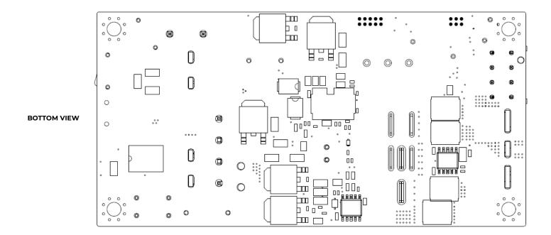
The CLP0205 is fastened to standard M3 pillars by standard M3 screws. We recommend a type with a captive anti-vibration washer, and here just as an example.
