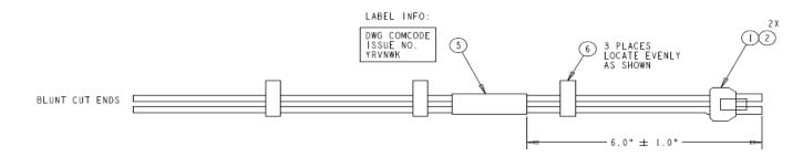
Wire 2 – DC Power output – example of similar lead for illustration purposes only (CLP0205 lead has 8 wires, due to its high output current)
