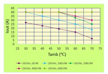
The CLP0205 is able to be used in a sealed enclosure, which also includes the load dissipation. As there are many different variables to be taken into account, each customer has to carry out their own thermal tests. As a general guide, OmniOn presents the derating curve for using CLP0205 in our sealed enclosure with OmniOn standard practice.
