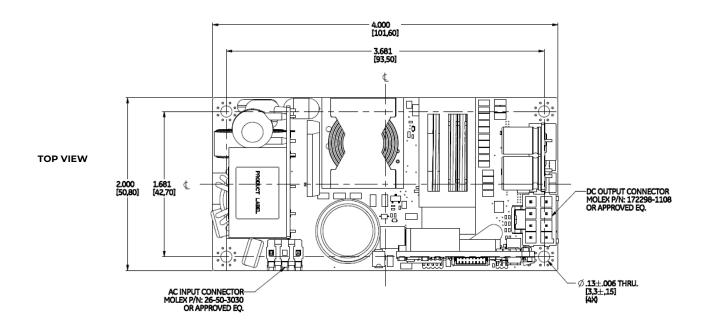
Mounting hardware is standard metric M3, and the mounting holes are 3.3 mm diameter.
