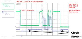
**Example waveforms showing clock stretching**
