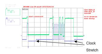
Figure 1. Example waveforms showing clock stretching.
