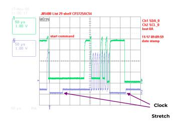
Figure 1. Example waveforms showing clock stretching.
