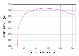
Figure 1. Converter Efficiency versus Output Current.
