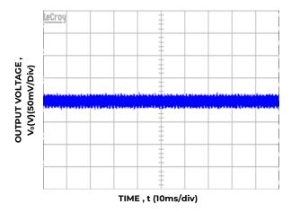
Figure 5. 12V output ripple and noise (  $V_{\text{in}}:\text{-48V}_{\text{dc}}$  , full load)
