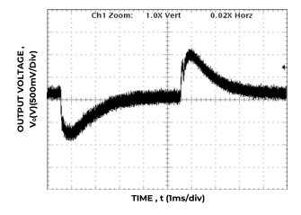
Figure 7. 12V Transient response load step 20–120A,  $V_{\text{IN}}$  = -48 $V_{\text{DC}}$
