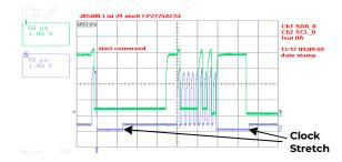
Figure 1. Example waveforms showing clock stretching
