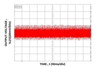
Figure 6. 3.3V output ripple and noise (  $V_{\text{in}}:\text{-}48V_{\text{dc}}$  , full load)
