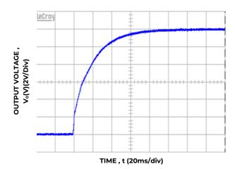
Figure 4.12V start-up ( $V_{in}$ : -48 $V_{DC}$ , full load)
