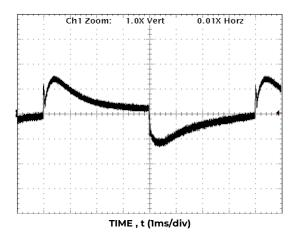
Figure 8. 12V Transient response 100 – 200A,  $V_{\text{IN}}$  = -48 $V_{\text{DC}}$
