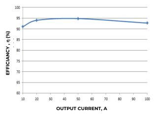
Figure 1. Converter Efficiency versus Output Current.
