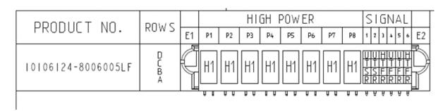
Short signal pins: F, H Long signal pins: R,S,T,U
