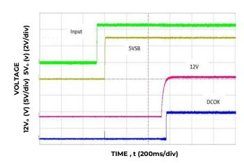
Figure 2. Input Start up (Vin: -48VDC, ful load)
