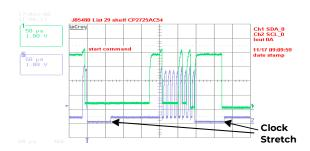
Figure 1 3.Example waveforms showing clock stretching
