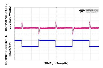
Figure 8. Transient response 12V<sub>DC</sub> output load step 50 - 100A,  $V_{IN} = -48V_{DC}$ .
