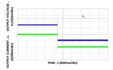
Figure 11. Overload: output short circuit performance, the unit is in latch\_OFF mode. ,  $V_{\text{IN}}$  = -48 $V_{\text{DC}}$ .
