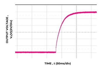
Figure 4. 12V start-up ( $V_{in}: -48V_{DC}$ , full load)
