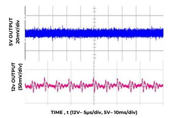
Figure 5. 12V output ripple and noise (  $V_{\text{in}}$  : -48 $V_{\text{dc}}$  , full load)
