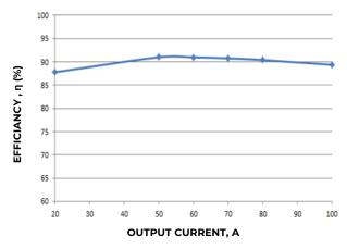
Figure 1. Converter Efficiency versus Output Current.
