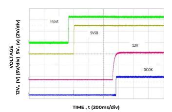
Figure 2. Input Start up (Vin: -48VDC, ful load)
