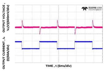
Figure 7. Transient response 12V<sub>DC</sub> output load step 10 - 60A, VIN = -48VDC.
