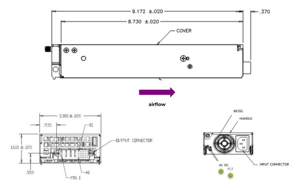
No handle, ac inlet – replace with wire extension with stress relief. 16ga -
