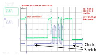
Figure 1. Example waveforms showing clockstretching.
