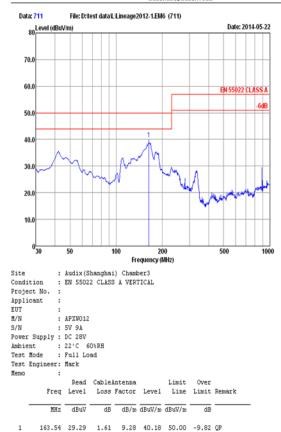
Fig 44 – EMI Plot of APXW012 on evaluation board with 28 V in in / 5 Vdc @ 9 A out
