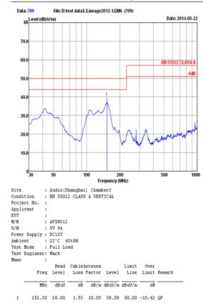
Fig 43 - EMI Plot of APXW012 on evaluation board with 12 V in, 5Vo @ 9 A out
