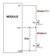
Figure 46. Circuit Configuration for margining Output voltage.
