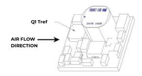
Figure 49. Preferred airflow direction and location of hot-spot of the module (Tref).
