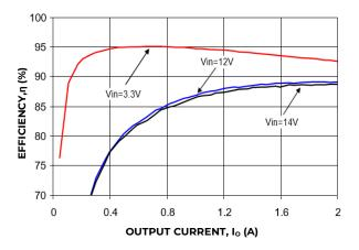
Figure 25. Converter Efficiency versus Output Current.
