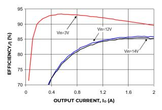
Figure 13. Converter Efficiency versus Output Current.
