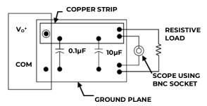
NOTE: All voltage measurements to be taken at the module terminals, as shown above. If sockets are used then Kelvin connections are required at the module terminals to avoid measurement errors due to socket contact resistance.
