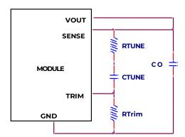
Figure. 47. Circuit diagram showing connection of RTUME and CTUNE to tune the control loop of the module
