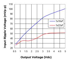
Figure 41. Input ripple voltage for various output voltages with 1x10 μF or 1x22 μF ceramic capacitors at the input (2A load). Input voltage is 12V.
