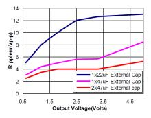
Figure 42. Output ripple voltage for various output voltages with external 1x22 μF, 1x47 μF or 2x47 μF ceramic capacitors at the output (2A load). Input voltage is 12V.
