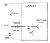
Figure 43. Circuit configuration for using negative On/Off logic.
