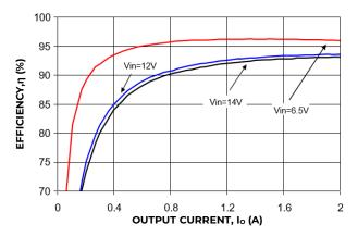
Figure 31. Converter Efficiency versus Output Current.
