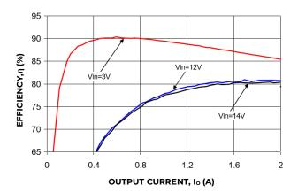
Figure 7. Converter Efficiency versus Output Current.
