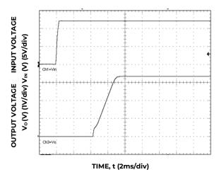
Figure 24. Typical Start-up Using Input Voltage (VIN = 12V, Cext=  $22\mu F$ , Io = Io,max).
