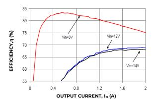
Figure 1. Converter Efficiency versus Output Current.
