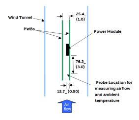
Figure 48. Thermal Test Setup.
