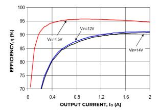
Figure 19. Converter Efficiency versus Output Current.
