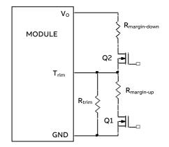
Figure 58. Circuit configuration for margining output voltage
