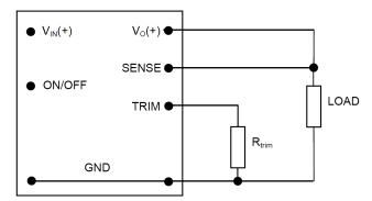
Figure 57. Circuit configuration to program output voltage using an external resistor
