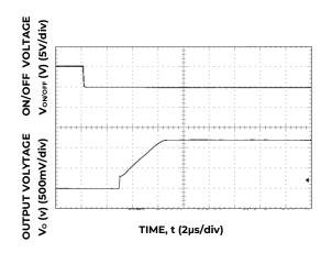
Figure 11. Typical Start-up Using On/Off Voltage (I₀ = I₀,max ,VIℕ = 8V).
