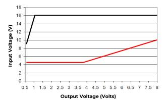
Figure 56. Output Voltage vs. Input Voltage Set Point Area plot showing limits where the output voltage can be set for different input voltages.
