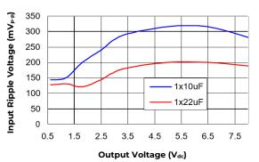
Figure 52. Input ripple voltage for various output voltages with 1x10  $\mu$ F or 1x22  $\mu$ F ceramic capacitors at the input (4A load). Input voltage is 12V.
