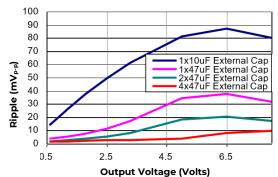
Figure 53. Output ripple voltage for various output voltages with 1x10 µF, 1x47 µF or 2x47 µF or 4x47 µF ceramic capacitors at the output (4A load). Input voltage is 12V.
