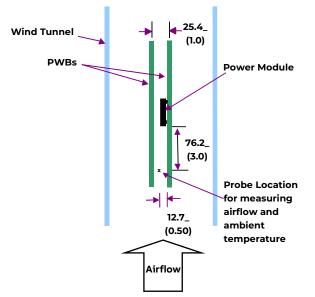
Figure 35. Thermal Test Set-up.
