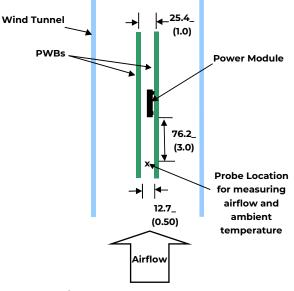
Figure 49. Thermal Test Set-up.
