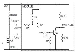
Figure 42. Circuit configuration for using positive logic On/Off logic.
