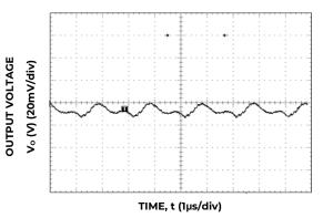
Figure 9. Typical Output ripple and noise (V<sub>in</sub> = 12V, I<sub>o</sub>=I<sub>o,max</sub>).
