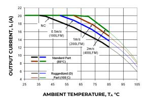
Figure 20. Derating Output Current versus Local Ambient Temperature and Airflow Ruggedized Part is discontinued
