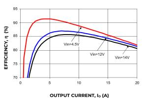
Figure 7. Converter Efficiency versus Output Current.
