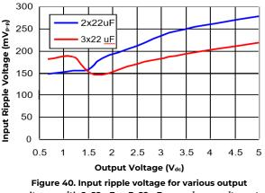
voltages with 2x22  $\mu$ F or 3x22  $\mu$ F ceramic capacitors at the input (20A load). Input voltage is 12V
