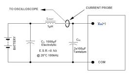
Figure 37. Input Reflected Ripple Current Test Setup.
