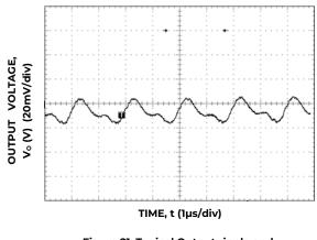
Figure 21. Typical Output ripple and noise, V<sub>IN</sub> = 12 V Io = Io, max.
