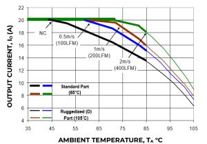
Figure 2. Derating Output Current verses Ambient Temperature and Airflow (Ruggedized Part is Discontinued)
