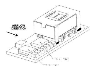
Figure 50. Preferred airflow direction and location of hotspot of the module (T<sub>ref</sub>).
