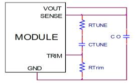
Figure. 48. Circuit diagram showing connection of RTUME and CTUNE to tune the control loop of the module.
