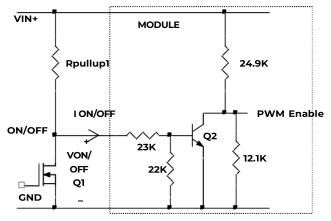
Figure 43. Circuit configuration for using negative logic On/OFF.
