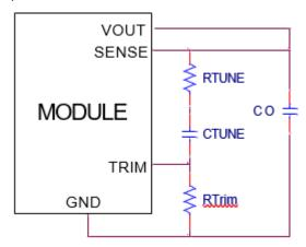
Figure. 48. Circuit diagram showing connection of  $R_{\text{TUNE}}$  and  $C_{\text{TUNE}}$  to tune the control loop of the module.
