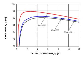
Figure 13. Converter Efficiency versus Output Current.
