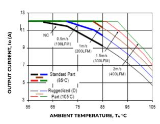
Figure 20. Derating Output Current versus Local Ambient Temperature and Airflow.
