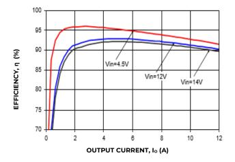
Figure 19. Converter Efficiency versus Output Current.
