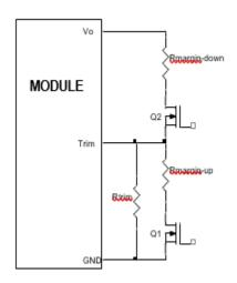
Figure 46. Circuit Configuration for margining Output voltage
