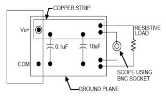
Figure 38. Output Ripple and Noise Test Setup.
