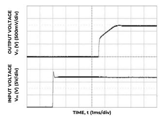
Figure 12. Typical Start-up Using Input Voltage  $(V_{\text{IN}} = 12V, \, I_o = I_{o,max}).$
