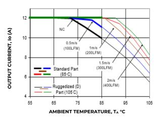
Figure 8. Derating Output Current versus Local Ambient Temperature and Airflow.
