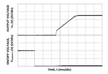
Figure 33. Typical Start-up Using On/Off Voltage ( $I_o = I_{o,max}$ ).
