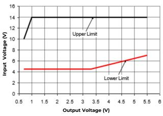
Figure 44. Output Voltage vs. Input Voltage Set Point Area plot showing limits where the output voltage can be set for different input voltages.
