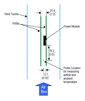
Figure 49. Thermal Test Setup.
