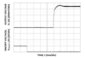
Figure 5. Typical Start-up Using On/Off Voltage (I $_{\rm o}$  = I $_{\rm o,max}$ ).
