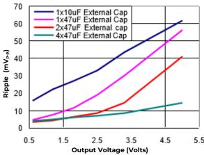
Figure 41. Output ripple voltage for various output voltages with external 1x10 µF, 1x47 µF, 2x47 µF or 4x47 µF ceramic capacitors at the output (12A load). Input voltage is 12V.
