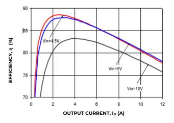
Figure 1. Converter Efficiency versus Output Current.
