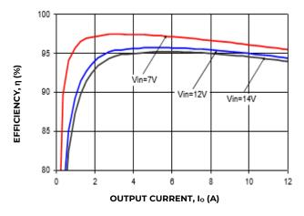
Figure 31. Converter Efficiency versus Output Current.
