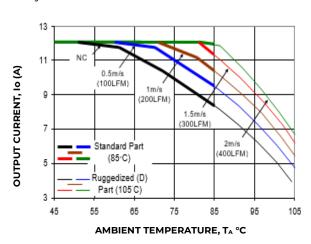
Figure 34 Derating Output Current versus Local **Ambient Temperature and Airflow.**
