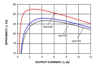
Figure 7. Converter Efficiency versus Output Current.
