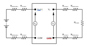
Figure 39. Output Voltage and Efficiency Test Setup.
