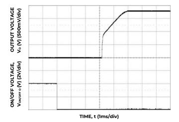
Figure 17. Typical Start-up Using On/Off Voltage  $(I_0 = I_{0,max})$ .
