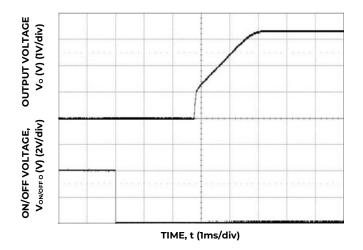
Figure 29. Typical Start-up Using On/Off Voltage ( $I_0 = I_{0,max}$ ).
