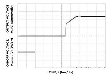
Figure 11. Typical Start-up Using On/Off Voltage ( $I_0 = I_{0,max}$ ).
