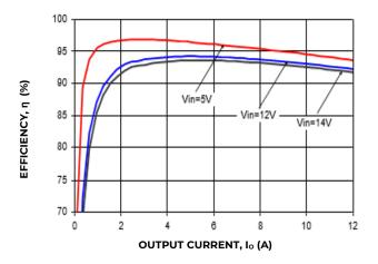
Figure 25. Converter Efficiency versus Output Current.
