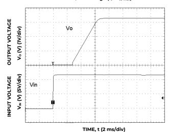
Figure 30. Typical Start-up Using Input Voltage ( $V_{IN} = 12 \text{ V } I_0 = I_{O, \text{ max.}}$ )
