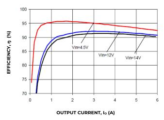
Figure 25. Converter Efficiency versus Output Current.
