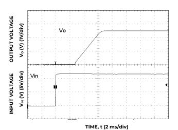
Figure 24. Typical Start-up Using Input Voltage ( $V_{IN} = 12 \text{ V } I_0 = I_{O, \text{ max.}}$ )
