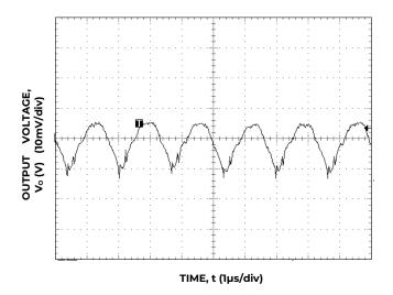
Figure 9. Typical Output Ripple and Noise,  $V_{IN} = 12 \text{ V } I_0 = I_0, \text{ max.}$
