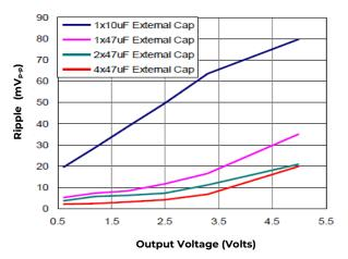
Figure 41. Output ripple voltage for various output voltages with external 1x10 μF, 1x47 μF, 2x47 μF or 4x47 μF ceramic capacitors at the output (6A load). Input voltage is 12V.
