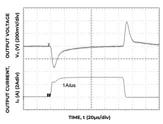
Figure 10. Transient Response to Dynamic Load Change from 50% to 0%.
