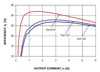
Figure 13. Converter Efficiency versus Output Current.
