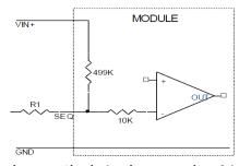
Figure 47. Circuit showing connection of the sequencing signal to the SEQ pin.
