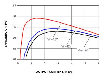
Figure 7. Converter Efficiency versus Output Current.
