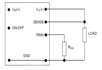
Figure 45. Circuit configuration for programming output voltage using an external resistor.
