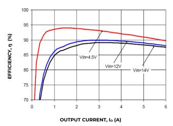
Figure 19. Converter Efficiency versus Output Current.
