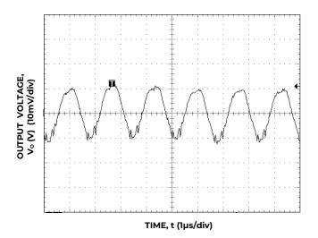
Figure 15. Typical Output Ripple and Noise,  $V_{IN} = 12 \text{ V } I_O = I_{O, \text{ max.}}$
