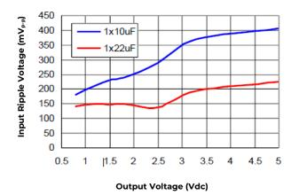
Figure 40. Input ripple voltage for various output voltages with 1x10  $\mu$ F or 1x22  $\mu$ F ceramic capacitors at the input (6A load). Input voltage is 12V.
