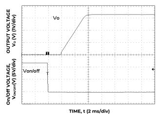
Figure 29. Typical Start-up Using On/Off Voltage (I<sub>o</sub> = I<sub>o</sub>, <sub>max</sub>).
