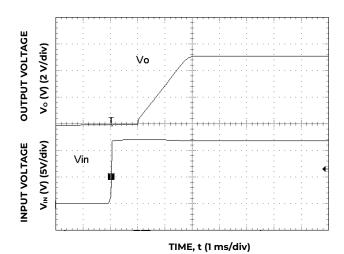
Figure 36. Typical Start-up Using Input Voltage ( $V_{IN} = 12 \text{ V } I_0 = I_{O, \text{ max.}}$ )
