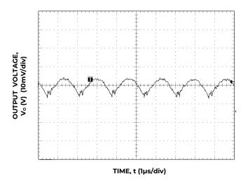
Figure 3. Typical Output Ripple and Noise,  $V_{IN} = 12 \text{ V I}_0 = I_0$ , max.
