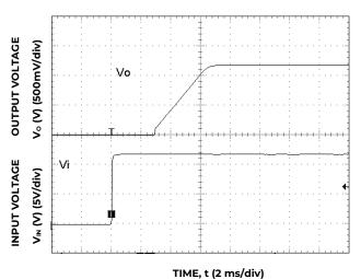
Figure 12. Typical Start-up Using Input Voltage ( $V_{IN} = 12 \text{ V } I_0 = I_0, \text{ max.}$ )
