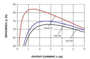
Figure 1. Converter Efficiency versus Output Current.
