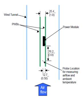
Figure 49. Thermal Test Setup.
