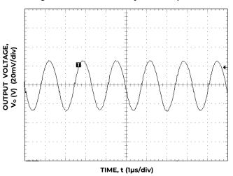
Figure 32. Typical Output Ripple and Noise, V<sub>IN</sub> = 12 V I<sub>O</sub> = I<sub>O</sub>, max.
