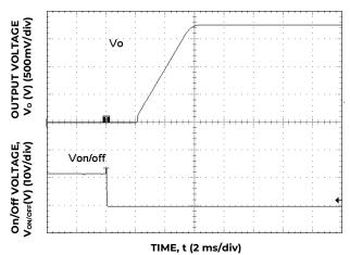
Figure 17. Typical Start-up Using On/Off Voltage ( $I_0 = I_0$ , max).
