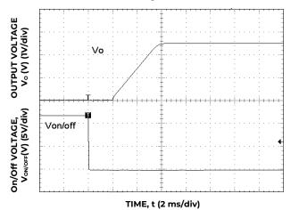
Figure 23. Typical Start-up Using On/Off Voltage ( $I_0 = I_0$ , max).
