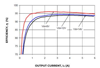
Figure 31. Converter Efficiency versus Output Current.
