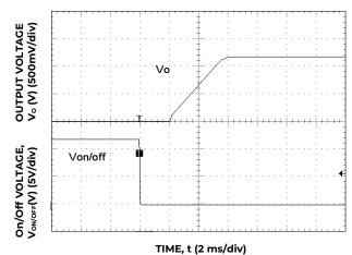
Figure 11. Typical Start-up Using On/Off Voltage ( $I_0 = I_0$ , max).
