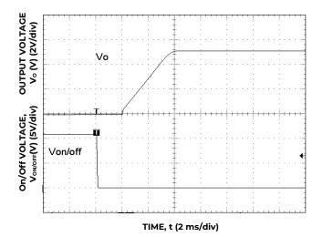
Figure 33. Typical Start-up Using On/Off Voltage (I<sub>o</sub> = I<sub>o</sub>, max).
