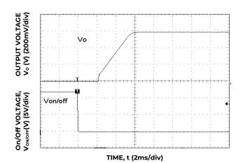
Figure 5. Typical Start-up Using On/Off Voltage (I<sub>o</sub> = I<sub>o</sub>, <sub>max</sub>).
