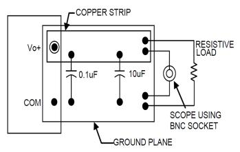
Figure 38. Output Ripple and Noise Test Setup.
