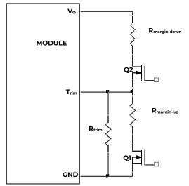
Figure 42. Circuit Configuration for margining Output voltage.
