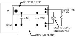
Figure 32. Output Ripple and Noise Test Setup.
