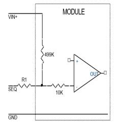
Figure 43. Circuit showing connection of the sequencing signalto the SEQ pin.
