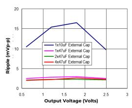
Figure 37. Output ripple voltage for various output voltages with external 1x10  $\mu$ F, 1x47  $\mu$ F, 2x47  $\mu$ F or 4x47  $\mu$ F ceramic capacitors at the output (6A load). Input voltage is 3.3V.
