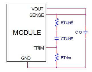
Figure. 44. Circuit diagram showing connection of  $R_{TUME}$  and  $C_{TUNE}$  to tune the control loop of the module.
