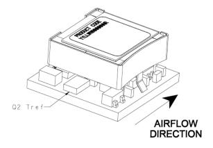
Figure 46. Preferred airflow direction and location of hotspot of the module (T<sub>ref</sub>).
