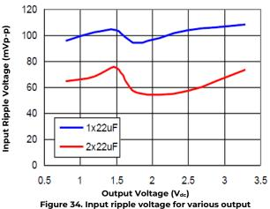
voltages with 1x22 µF or 2x22 µF ceramic capacitors at the input (6A load). Input voltage is 5V
