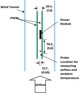
45. Thermal Test Setup.
