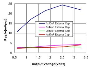
Figure 36. Output ripple voltage for various output voltages with external 1x10 μF, 1x47 μF, 2x47 μF or 4x47 μF ceramic capacitors at the output (6A load). Input voltage is 5V.
