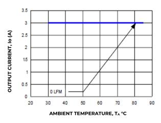
Figure 26. Derating Output Current versus Local Ambient Temperature and Airflow.
