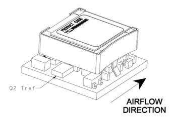
Figure 45. Preferred airflow direction and location of hotspot of the module ( $T_{\rm ref}$ ).
