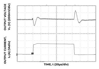
Figure 22. Transient Response to Dynamic Load Change from 0% to 50% to 0%. With  $V_{\text{IN}}$  = 5V
