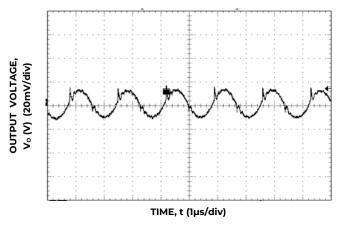
Figure 21. Typical output ripple and noise ( $V_{IN}$  = 5V,  $I_o$  =  $I_{o,max}$ ).
