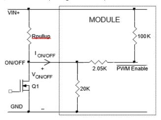
Figure 38. Circuit configuration for using negative On/Off logic.
