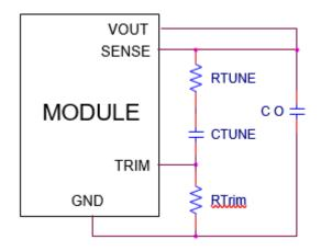
Figure. 43. Circuit diagram showing connection of  $R_{\text{TUNE}}$  and  $C_{\text{TUNE}}$  to tune the control loop of the module.
