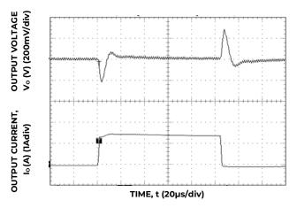
Figure 28. Transient Response to Dynamic Load Change from 0% to 50% to 0%. With  $V_{\text{IN}}$  = 5V
