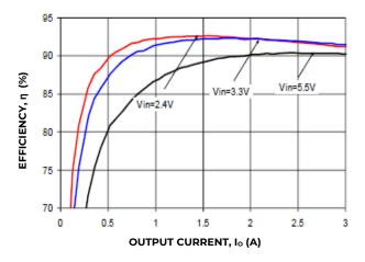
Figure 13. Converter Efficiency versus Output Current.
