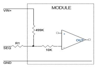
Figure 42. Circuit showing connection of the sequencing signal to the SEQ pin.
