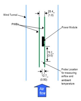
Figure 44. Thermal Test Setup.
