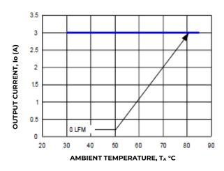
Figure 14 Derating Output Current versus Local Ambient Temperature and Airflow.
