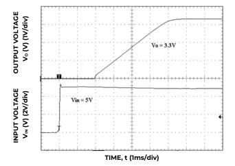
Figure 30 Typical Start-up Using Input Voltage  $(V_{\text{IN}} = 5V, \ I_{\text{o}} = I_{\text{o,max}}).$
