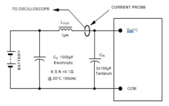
Figure 31. Input Reflected Ripple Current Test Setup.
