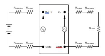
Figure 33. Output Voltage and Efficiency Test Setup.
