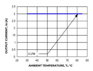
Figure 2. Derating Output Current versus Local Ambient Temperature and Airflow.
