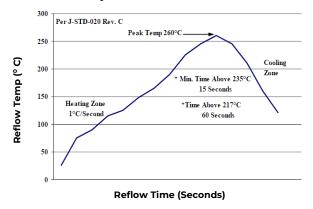
Figure 46. Recommended linear reflow profile using Sn/Ag/Cu solder.
