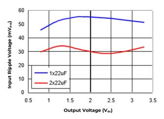
Figure 34. Input ripple voltage for various output voltages with  $1x22~\mu F$  or  $2x22~\mu F$  ceramic capacitors at the input (3A load). Input voltage is 5V.
