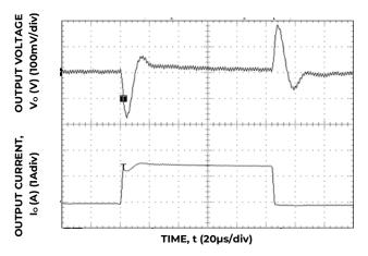
Figure 10. Transient Response to Dynamic Load Change from 0% to 50% to 0%. With  $V_{\text{IN}}$  = 5V
