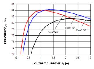
Figure 1. Converter Efficiency versus Output Current.
