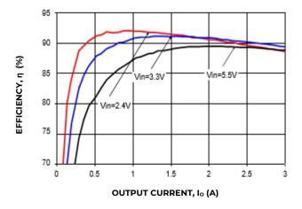
Figure 7. Converter Efficiency versus Output Current.
