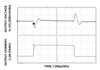
Figure 16. Transient Response to Dynamic Load Change from 0% to 50% to 0%. With  $V_{\text{IN}}$  = 5V
