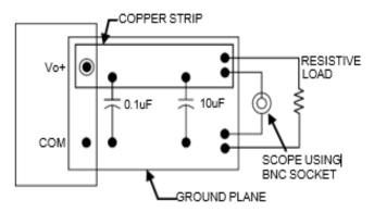
Figure 32. Output Ripple and Noise Test Setup.
