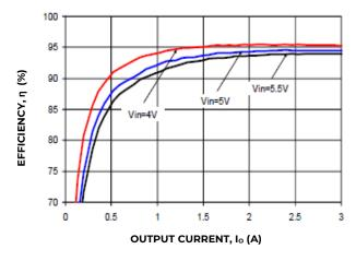
Figure 25. Converter Efficiency versus Output Current.
