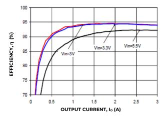
Figure 19. Converter Efficiency versus Output Current.
