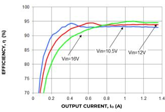
Figure 13. Converter Efficiency verses output current
