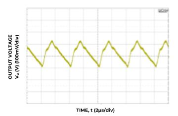
Figure 3. Typical output ripple ( $C_0=66\mu$ F ceramic,  $V_{IN} = 12V$ ,  $I_0 = I_{0,max}$ ,).
