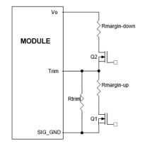
Figure 31. Circuit Configuration for margining Output voltage.
