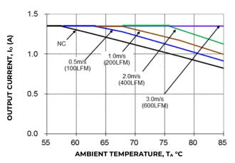
Figure 14. Derating Output Current verses Ambient Temperature and Airflow. Vin = 12V
