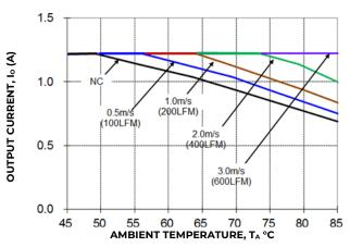
Figure 20. Derating Output Current verses Ambient Temperature and Airflow, VIN = 12V
