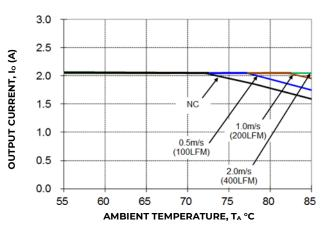
Figure 2. Derating Output Current verses Ambient Temperature and Airflow. Vin = 12V
