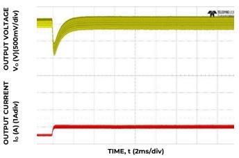
Figure 22. Transient Response to Dynamic Load Change from 0.6 to 1.1A at 12Vin, Cout= 7x4.7uF CTune=82pF, RTune=40.2Ω
