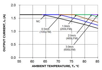
Figure 8. Derating Output Current verses Ambient Temperature and Airflow. VIN=12V
