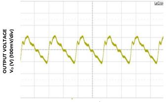
TIME, t (2μs/div) Figure 9. Typical output ripple and noise (Co=66μF ceramic, V<sub>IN</sub> = 12V, Io = Io,max, ).
