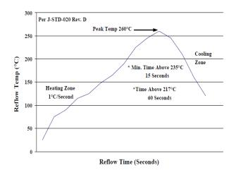
Figure 35. Recommended linear reflow profile using Sn/Ag/Cu solder.
