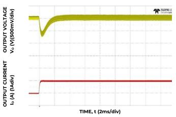
Figure 4. Transient Response to Dynamic Load Change from 50% to 100% at 12Vin, Cout= 12x4.7uF, CTune=820pF, RTune=30.1\Omega
