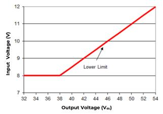
Figure 30. Output Voltage vs. Input Voltage Set Point Area plot showing limits where the output voltage can be set for different input voltages.
