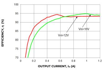
Figure 19. Converter Efficiency verses output current
