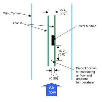
Figure 33. Thermal Test Setup.
