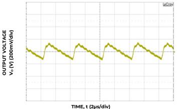
Figure 21. Typical output ripple and noise (Co=66 $\mu$ F ceramic, V<sub>IN</sub> = 12V, Io = Io,max, ).
