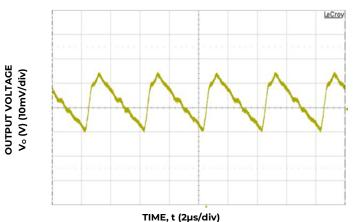
Figure 15. Typical output ripple and noise (Co=66µF ceramic,  $V_{IN}$  = 12V, Io = Io,max, ).
