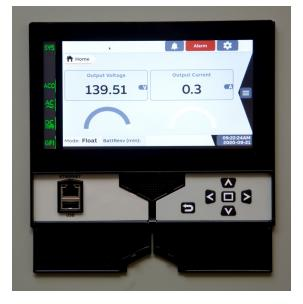
Nebula is the latest embedded controller in the Integritas<sup>™</sup> family of products with advanced system monitoring and control features. Built on a modern ARM based platform, the controller monitors system components within the charger including rectifiers, inputs, outputs, and alarms utilizing a high speed digital communications bus.
