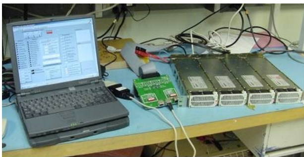
Figure 10 -Test setup using a OmniOn J85480 shelf
