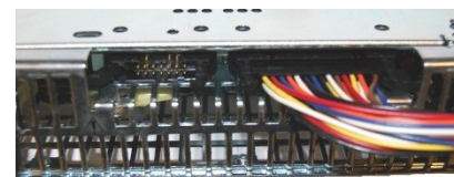
Figure 14 - Control cable plugged into the J1 connector
