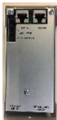
Figure 9 VIM1EC Meter RS485 Connection
