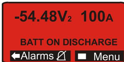
The audible alarm may be disabled altogether through proper configuration at the front panel or through remote means.
