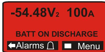
Pressing the arrow key on a Pulsar controller or the ACO pushbutton on a Phoenix controller provides a quickly temporarily silences the audible alarm.
