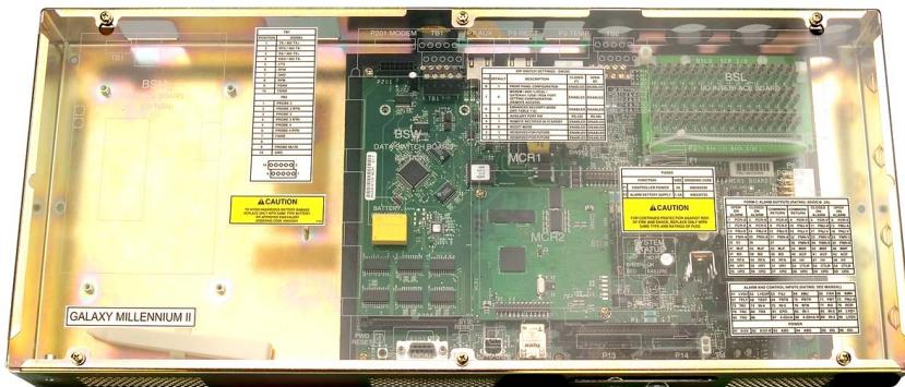
Capable of controlling and monitoring as many as 64 rectifiers, the GALAXY MILLENNIUM II Controller simplifies the administration and surveillance associated with power plants and auxiliary equipment.
