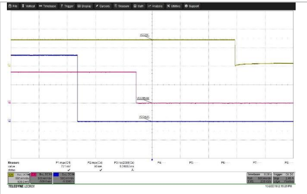
Figure 4 – OFF Sequence – VCCINT (Yellow), VCCBRAM(Red), VCCAUX(Blue) (Axis Scale : 500mV(y), 500ms(x))
