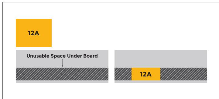
This low-profile power solution also comes into play when placing a separate open-frame power module on a secondary PCB “daughter” board. Again, SlimLynx can be placed below the PCB or on the “mezzanine” between the main and secondary board, freeing up valuable space and height for additional components.
