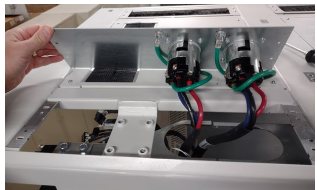
Figure 7 AC panel removed
