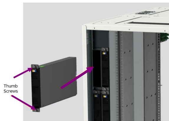
Figure 30 Rectifier Module Installation
