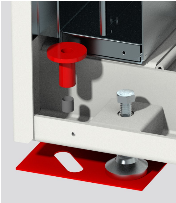
Figure 9A EDGE Isolation Plate Kit - 1600305789A
